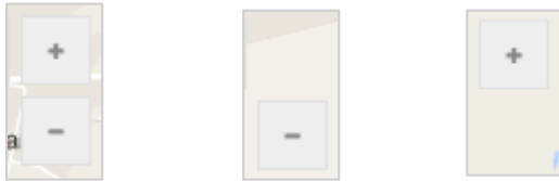
Figure 10 - Zoom controls, Left: Both visible and most zooms, Middle: Zoom-in control hidden at max zoom, Right: Zoom-out control hidden at min zoom
